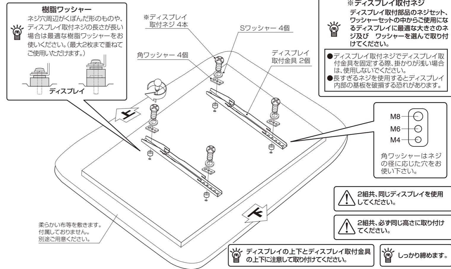
**6 ディスプレイの取付**
